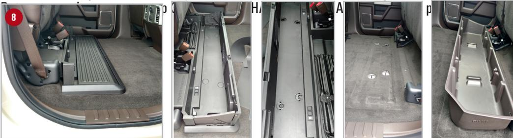
9 Some models of trucks have a vinyl floor and do not have the factory divider. To install the DU-HA in this type of truck set the DU-HA under the rear seat and position it so the slots are facing the back of the truck and line up with the larger middle hole and slot in the seat brackets. Next use the provided M6 knobs, M6 washers and M6 nuts to secure the DU-HA to the seat brackets.
